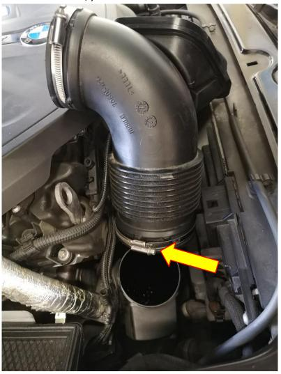
5. Take FMINLH25 and place a hose clamp to the end with the longer leg length. Now attach that end of the hose to the OEM turbo inlet. It should be angled as shown below.
