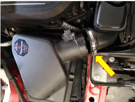
4. Using a 6mm socket and suitable drive undo the bottom of the OEM inlet hose where it attaches to the OEM turbo inlet, you can now remove the OEM inlet hose.
