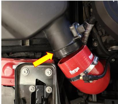
8. Attach FMINLH25 to the upper airbox and tighten the hose clamps accordingly at the airbox AND turbo inlet end of FMINLH25.
