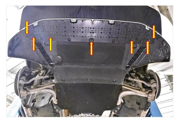
10. You will now be able to pull the sides of the bumper away from the wings and then the whole bumper will come away from the vehicle. IMPORTANT: do not pull the bumper fully from the vehicle till step 11 has been completed!
