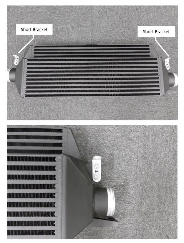
20. Place the intercooler into position, the lower mounting pegs on FMINT26 locate in the same position as the OE intercooler. Now replace the crash bar back into position.
