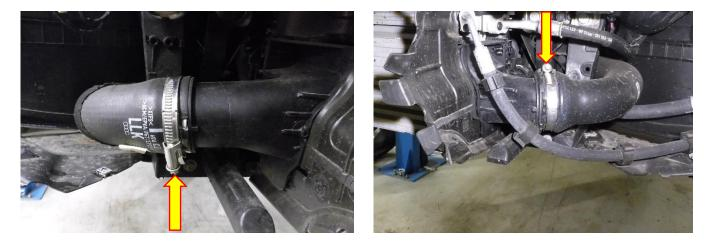
**17**. Using a flat blade screwdriver or trim tool press in the locking tabs for the intercooler ducting X2 on each side, then pull the ducting from the vehicle. **IMPORTANT: Do not re-fit ducting.**
