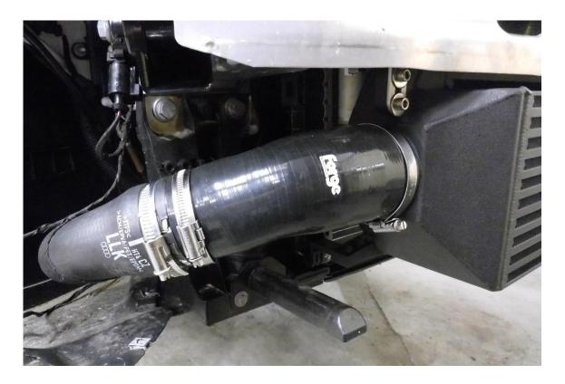
23. Take the remaining hose joiner, hose **#2052** and hose clamps and install them in the same way to the other side of the intercooler.
