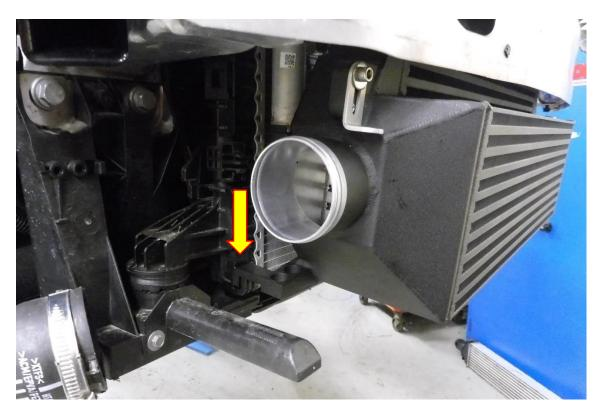
21. Using a 5 mm Allen key fit the remaining M6 fastener to the braket and intercooler. Mark the crash bar using a marker pen were to fastern the supplied tek screws to mount the intercooler to the crash bar. Alternitivly remove the crash bar once marked and Using a 4mm drill bit drill a hole in the marked location on the crash bar, then using an 8mm socket and ratchet attach the intercooler to the crash bar with the supplied self tapping fasteners.
