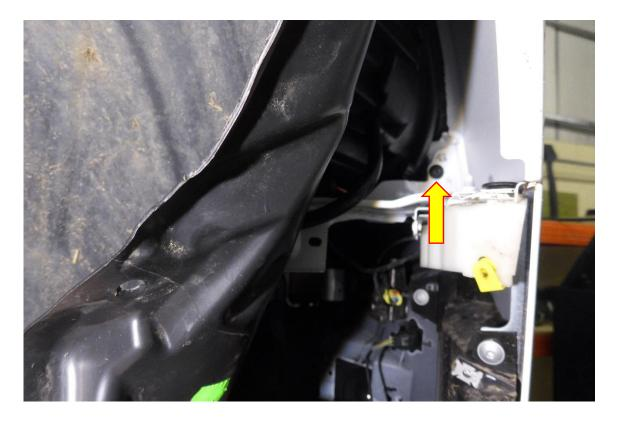
8. Using a trim tool remover or flat blade screw driver remove the plastic retaining fasteners attaching the top of the bumper to the wing on both sides of the vehicle.
