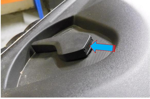
2. Using a trim removal tool prise the corner of the slam panel cover to allow your hand to get underneath it, then pull the front section upwards to release all the mounting clips. Now pull the cover towards you to remove it completely.
