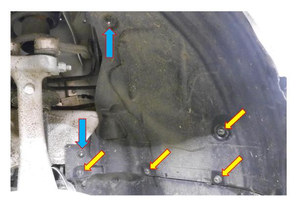
7. Peel back the arch liner and using a T30 Torx driver remove the fastener on both sides of the vehicle.
