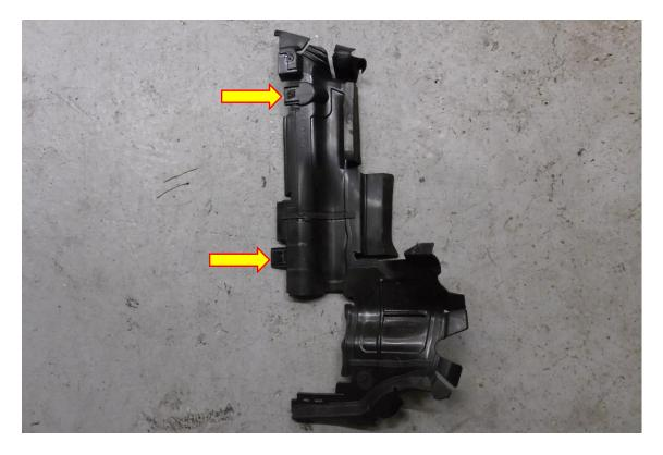
**18**. Using some long nose plyers press in both locking tabs at the top of the intercooler, you will now be able to pull the intercooler from the vehicle.
