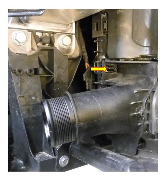
19. Take both the supplied brackets and X3 M6 Allen cap fasteners and washers from the FMINT26 kit then using a 5mm Allen key attach the short bracket to the left side of the intercooler but only fit one of the M6 fasteners at this stage and the longer bracket to the right side of the intercooler using X2 M6 fasteners.
