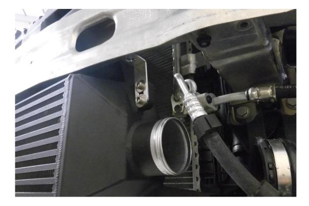
22. Take the 60mm hose joiner from the FMINT26 kit and fit it to the hot side boost pipe. Now attach hose#2051 for FMINT26 kit to the intercooler and hose joiner and secure them with hose clamps 50-70mm and 60-80mm.
