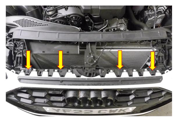
4. Using a T25 Torx drive remove the X4 fasteners attaching the edge of the wheel arch liner to the bumper on both sides of the vehicle.
