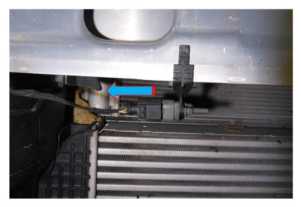
14. Using a 13mm socket and ratchet and a 13mm spanner remove the M8 nut and bolt's attaching the crash bar to the vehicle.
