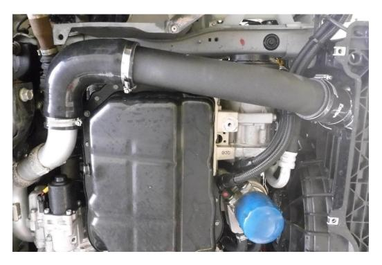
17. Now fit the near-side hose to the intercooler. This is also secured with 7mm hose clamps, the same as the off-side hoses.
