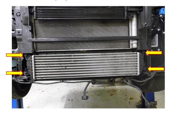
12. The rest of the off-side intercooler hose can be taken off the car, loosen the 8mm hose clamp in the same way as before, then undo the fastener holding the OE hard pipe to the car with a 10mm socket and rachet drive. Now remove the hose and pipe as one, from the vehicle.
