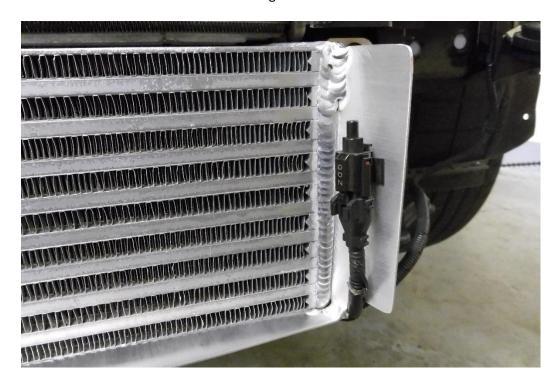
**15**. Using an angle grinder or hack saw, cut off the temperature sensor bracket, we recommend painting over the cut mark to prevent rusting.
