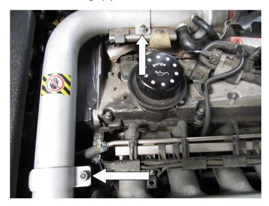
4/ Loosen off the hose clamp on the turbo hose **so that the hose can freely move round**. You may need to open the poppers on the heat shield.
