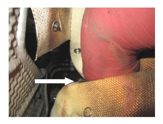
5/ Refit the new de-resonated charge pipe fitting the turbo end first then twisting it so that it fits perfectly in the locating brackets.
