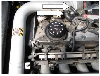
3 Undo the two 13mm nuts shown and remove the brackets.
