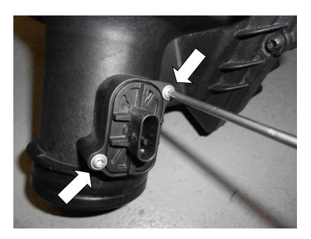
28. Fit the MAF sensor to your Forge Alloy induction pipe and secure using the 2x M3x12mm Allen cap bolts. The Arrow on the sensor pointing towards the engine.
