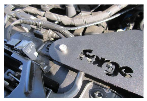
7. Using the two M8 fasteners place them through the induction tray putting the penny washers underneath followed by the two M8 nuts and secure in place.
