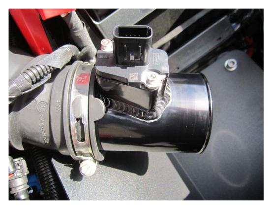
11. Now using your hose clamp driver fit the new high flow forge motorsport filter on to the end of the MAF housing .
