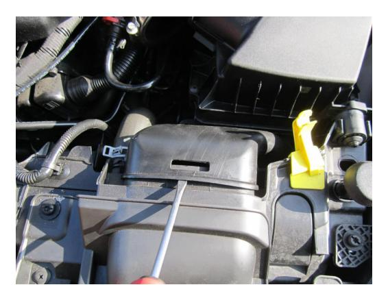
4. Now pull the airbox upwards to remove it from the rubber grommets that hold it place.
