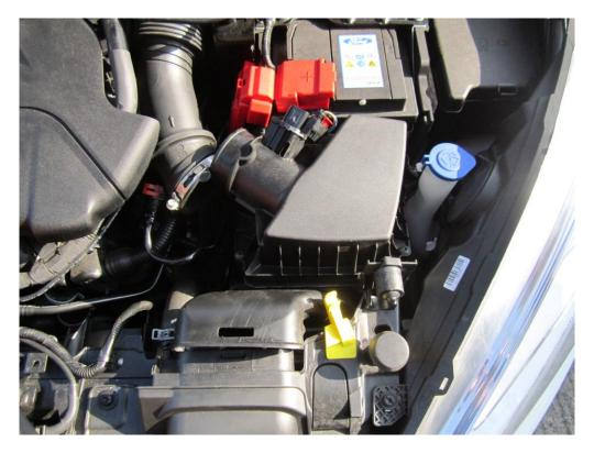
5. Now with the airbox removed place the new Forge Motorsport induction tray into position.
