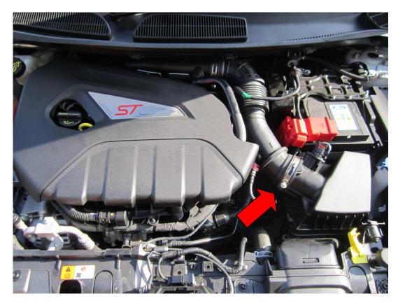
2. Now unclip the wiring loom from your MAF sensor, pull back the retaining clip that holds it in place then pull the loom away from the MAF sensor itself.
