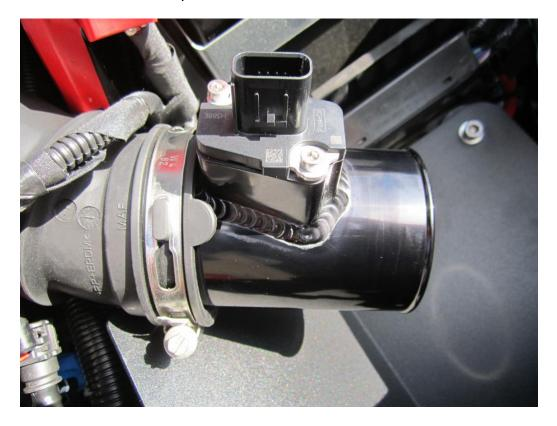
Now using your hose clamp driver fit the new high flow forge motorsport filter on to the end of the MAF housing .
