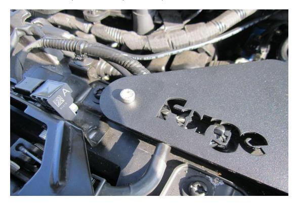
Using the two M8 fasteners place them through the induction tray putting the penny washers underneath followed by the two M8 nuts and secure in place.
