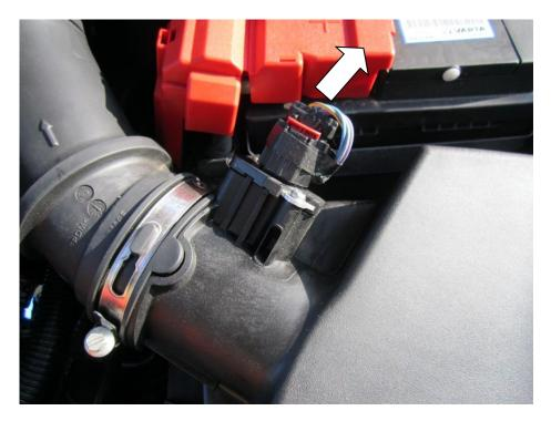
**3.** Using a flat bladed screwdriver pry the duct over the locater on the slam panel.
