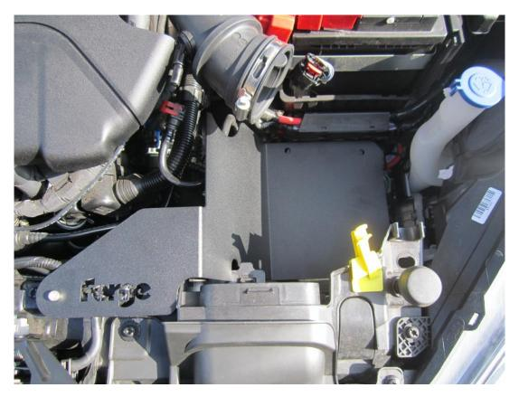
6. Using the M6 fastener provided, place the fastener through the induction tray and bolt to your slam panel .
