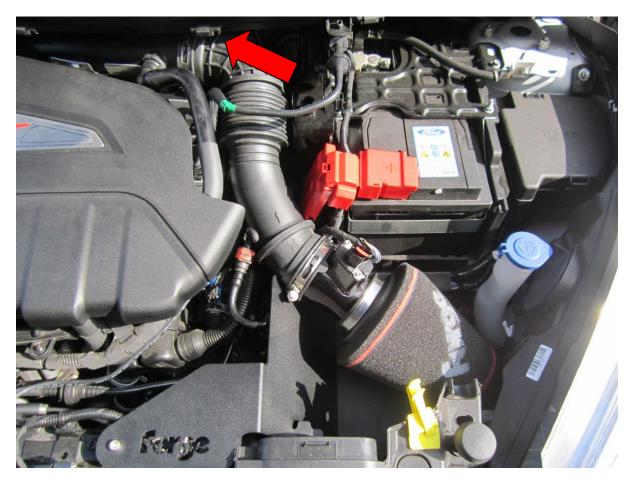
**12.** You may need to loosen the hose clamp arrowed red in the picture above and re-position the intake hose so it fits snugly into the induction tray, then re-tighten.
