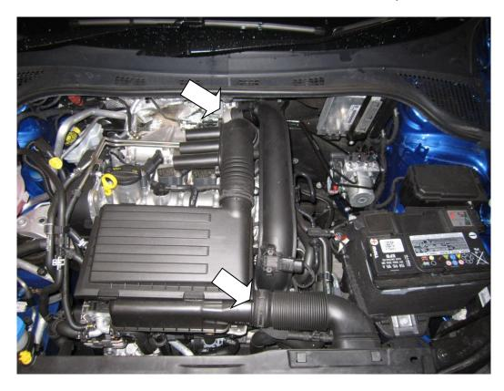
2. Now remove the inlet hose from its position by pushing down on the retaining clips as pictured below.
