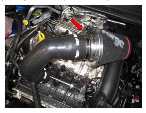
6. Fit the new silicon inlet hose into postion and connect the breather pipe to the rocker cover, then tighten the hose clamp.
