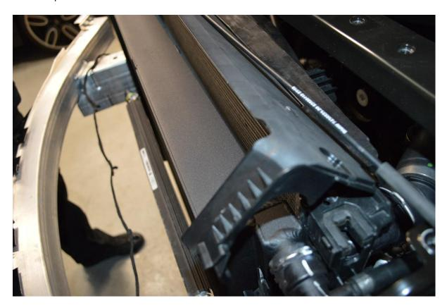
24. Mount the PAS cooler to the FMCCRAD12 to the machined bosses, use the two machined plates and four M5 fasteners to attach the PAS cooler in firmly place.
