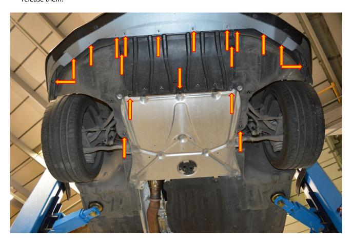
4. Locate the six M8 fasteners that attach the bumper to the wheel arch liners, remove these with an 8mm socket and ratchet.
