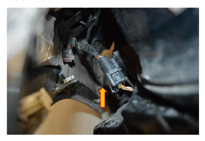
6. Unclip the loom to the pedestrian crash protection system, there is a plug on both sides that needs to be unclipped. Now remove the foam cover from the crash bar.
