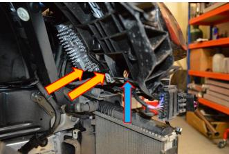
10. Remove the plastic slam panel, there are four M10 fasteners attaching this to the vehicle, use the relevant socket and ratchet to remove them.
