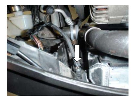
16. Disconnect the bonnet pull cable. The junction box is above the left-hand headlight. Open the junction box and disconnect the cable. <u>Ensure this is reattached correctly when</u> reassembling the vehicle otherwise you will be unable to reopen the bonnet.
