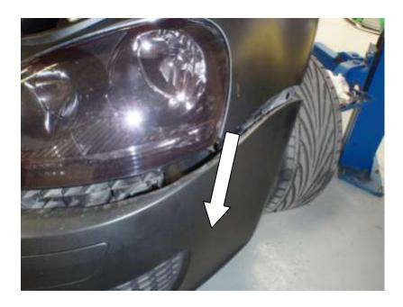
8. This next part requires two people, the first to hold the bumper while the second disconnects the wiring running to both fog lamps.
