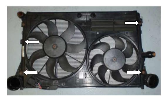
27. Unscrew the 4x T25 Torx screws on the back of the intercooler connecting the intercooler to the radiator. The Intercooler can now be carefully removed from the radiator and A/C radiator.
