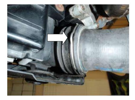
24. On the standard intercooler remove the standard rubber mount from each end. These are reused to mount your new Forge Intercooler.
