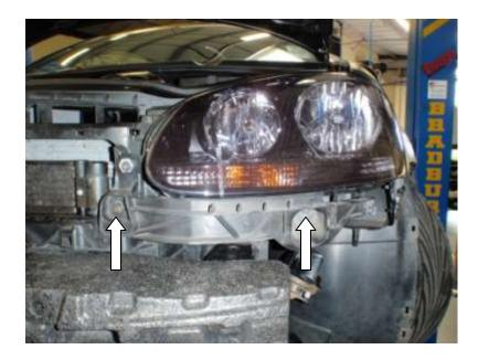
13. To release the headlight unit, undo 3x T25 Torx screws. Place in a safe place, away from the car to prevent damage while working on the rest of the car.
