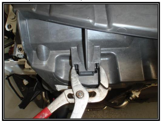
16. Reattach the radiator pack crash bar and bonnet catch in reverse order as shown in step 9, 10 and 12. Place the OEM intercooler blanking plate supplied into position using the bottom edge and right hand edge as a guide.
