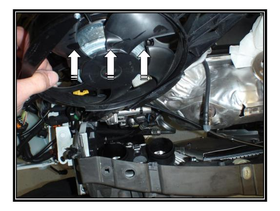
15. To remove the intercooler there is a clip in the front of the radiator pack, squeeze the clips together and push the intercooler towards the engine. You will need to pull the radiator pack forwards as much as possible to remove the intercooler.
