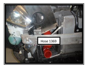
18. Fit the silicon hose to the boost pipe that leads to the inlet manifold. Position the intercooler so that the silicon hose is in the centre of the hole. To achieve this you will need to cut away some of the ducting for the outlet. Please see photos A and B.
