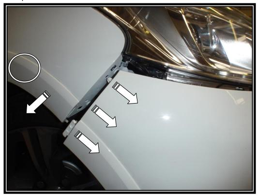
8. Undo three bolts, unclip the wiring and remove the lights.
