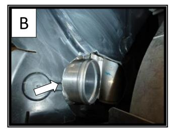
19. With the ducting cut and the intercooler in position use the nut driver bit supplied and the self-tapping screws with washers to secure the top of the intercooler. Then drill through the bottom brackets into the under tray with a 7mm drill and secure with the M6 bolts supplied in the kit. (Large washers must be used front and back)
