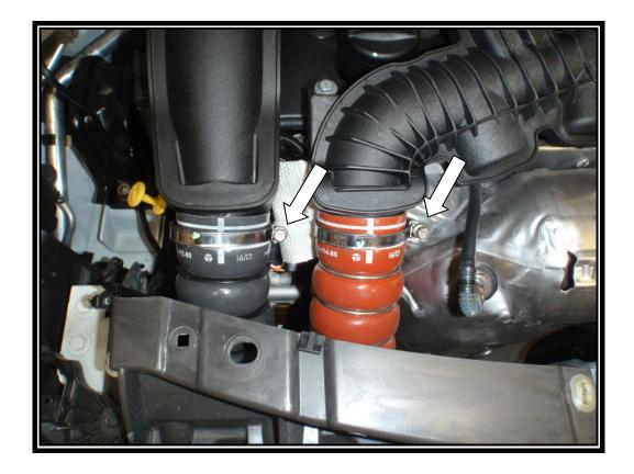
13. Undo the hose clamps on the top of the intercooler and remove the flexible hoses. Remove the screws holding the fan in position and unclip the radiator over flow pipe.
