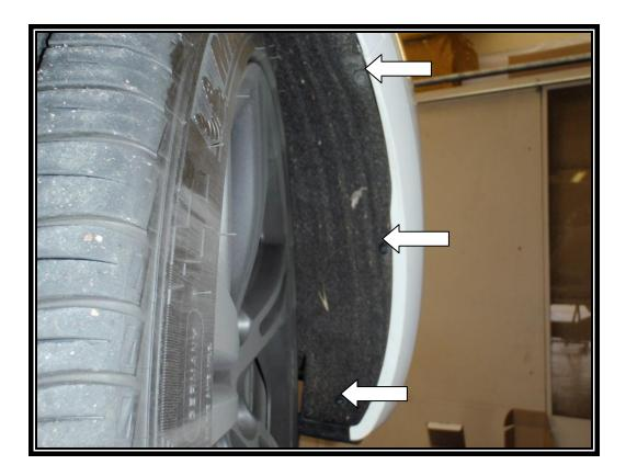
2. Using a flat bladed screw driver unclip and remove the plastic clips on the bottom edges of the bumper.
