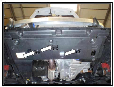
21. Position the hard pipe so that the slotted brackets are in line with the threaded holes. Please insure that hose 1368 is fitted in a position so that it is clear of the radiator. The bottom part of under tray has been dropped down only for visual reference on boost pipe position.
