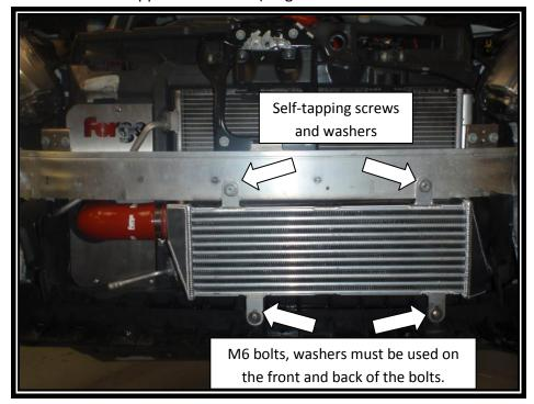
20. Remove the three bolts on the under tray. Position the aluminium boost pipe so that the brackets are sandwiched between the two parts of the under tray and the slots line up with the holes. Re fit the bolts and tighten please see step 21 for a clearer view.
