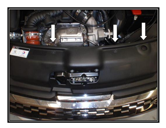
7. Behind the arch there is a small plastic clip squeeze the sides in and push the arch trim outwards. Pull the bumper down and forwards to release from the wings. The bumper is now free to remove.
