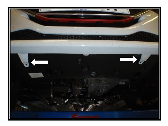
4. Undo the bolts holding the bumper to the wing, view is from inner arch.
