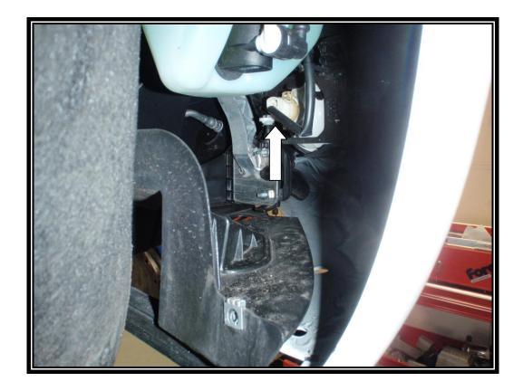
6. Moving to the top of the bumper unscrew the torx and remove the plastic clip.
