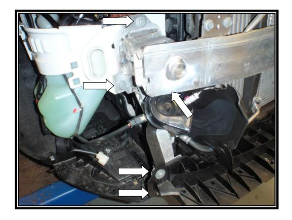
11. Remove the bolts at both ends of the radiator pack, lift up the radiator pack and pull forwards to gain access to the OEM intercooler and fan.
