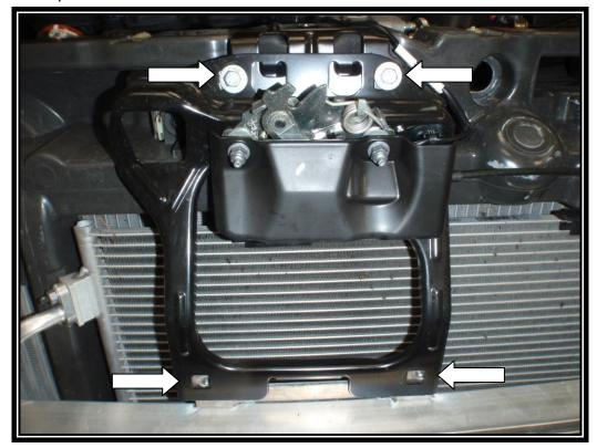
10. Undo the two bolts either side of the lower of crash bar, undo the six bolts either side at the top of the crash bar unclip the plastic under tray and remove.
