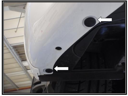
3. Undo the two bolts under the front bumper
