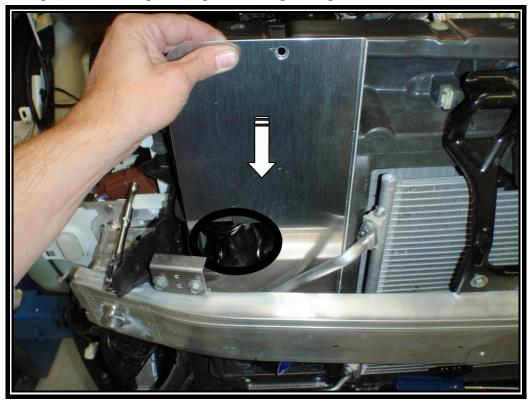
17. Drill through the three holes using a 4mm drill bit as shown below. Lift the plate out and insert hose 1369. Drop the plate back down and push the hose through the hole. Attach using the coarse threaded screws supplied in the kit.
