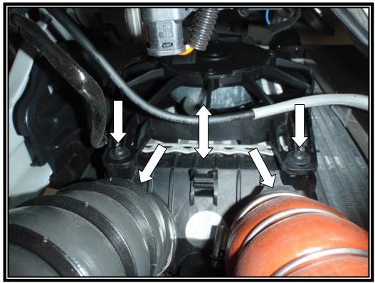
14. Lift the fan up and out of the engine bay, unclip the wiring and remove.
