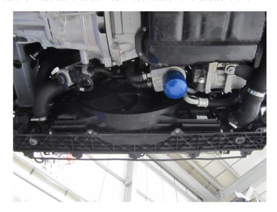
**12**. Finally, to remove the intercooler undo the 4 fasteners attaching it to the car, remove them using a 10mm socket and rachet drive. The intercooler can now be removed from the vehicle.
