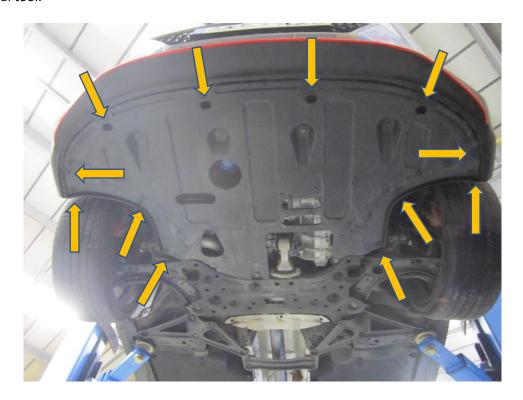
4. There are now 7 fasteners left holding the belly pan in place, remove all of these with a 10mm socket and rachet drive and slide it towards the front of the car to remove it.
