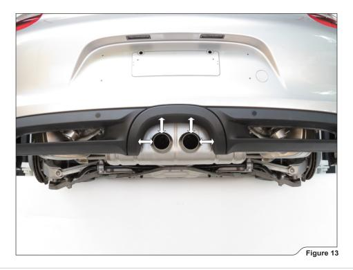
7. Tighten the muffler's brackets clamps and link pipes - muffler joints clamps on both sides of the vehicle (Figure 14).
