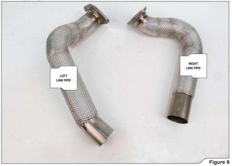
**!** WARNING: make sure, that you insert the link pipes all the way into the muffler's inlet pipes – use rubber mallet if necessary to tap the connections into place (Figure 10)!
